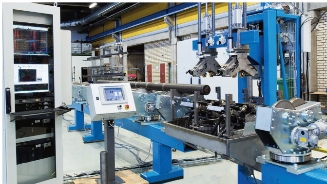
Echomac® Full Body Ultrasonic Test System for Spinning Tube. Echomac instrument controls are at left, powered roller head is at right, and APC carriers are shown in the middle as the tube approaches.
