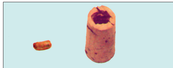
Ferrous filings are embedded in paraffin wax, shown above at left, then inserted in a hollowed out cork to create a calibration standard that can be inserted in the tube to be tested.
