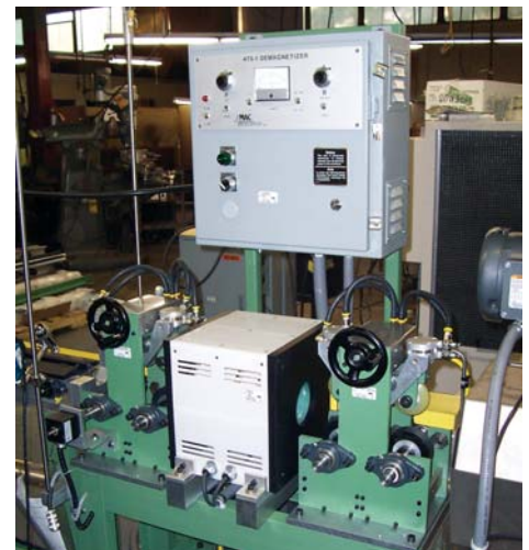
476 Demagnetizer and electronics on a "V" Roll Guide bench
