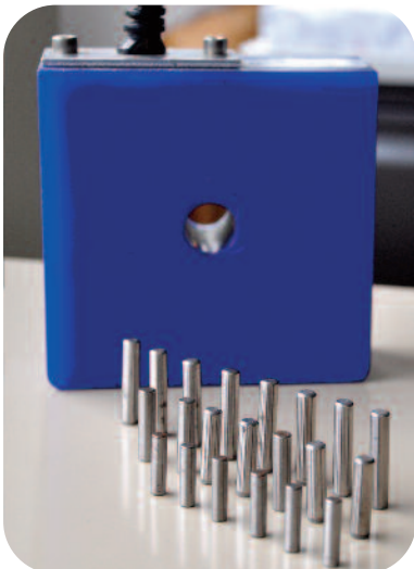
A typical eddy current test coil and .75", 1.00", and 1.25" long steel pins used to produce the test signals in the screen shown at upper right.
